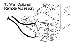
Figure 41 - Control Valve Terminals
